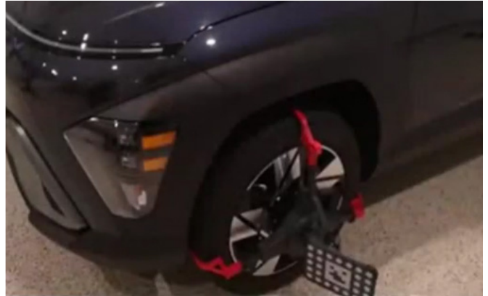
Figure 1: Targeted wheel clamps aid the IA1000 to perfectly position camera pattern to vehicle for precise calibrations
