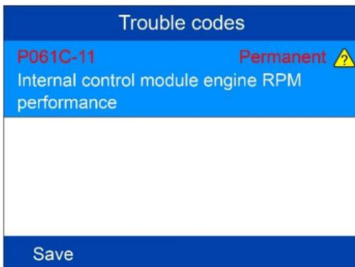
**Figure 3-10 Sample Engine Trouble Codes Screen**
