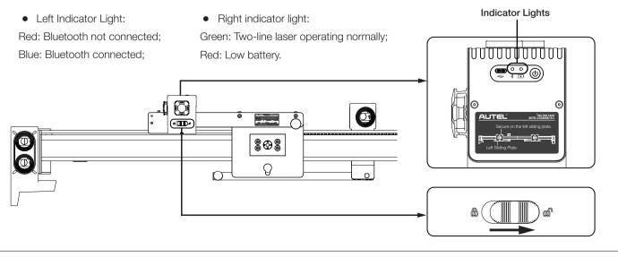
Check if the two-line laser is working properly: When the two-line laser is on, press the top button to activate or deactivate the laser. Hold the button for 4 seconds to put the laser into standby mode. If activated, the laser will automatically stop emitting after 5 minutes and enter standby mode after 10 minutes.
