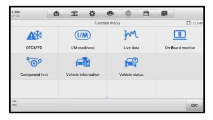
Figure 4-14 OBDII Diagnostics Menu Screen
