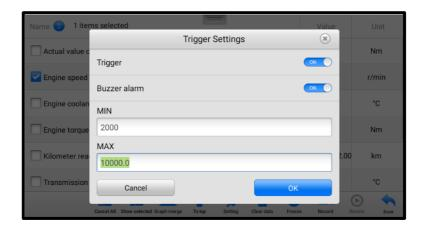
Figure 4-13 Trigger Setting Screen
