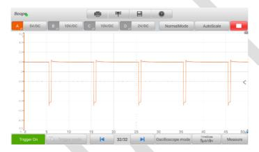
Figure 18-2 Square Waveform Screen
