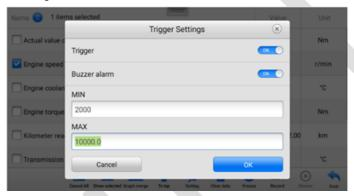
Figure 6-6 Trigger Setting Screen
