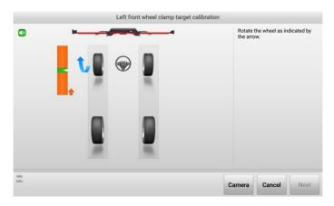
Figure 5-32 Start Calibration (Use Vehicle) 3
