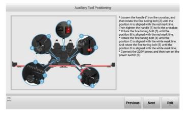
Figure 5-52 Auxiliary Tool Positioning 2
