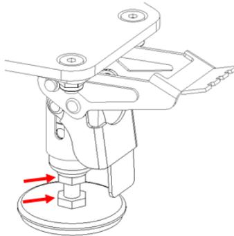
Adjustment method: use 2 monkey wrenches to snap into the two nuts on the bottom of the footbrake and loosen the upper nut in a clockwise direction, then rotate the foot cup to adjust to a suitable height. After that, rotate the upper nut in an anticlockwise direction to tighten the footbrake.
