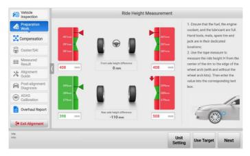
Figure 4-30 Measure Ride Height with Tape 1
