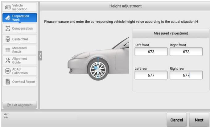
**Figure 4-27 Height Adjustment Screen 3**
