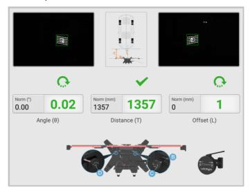
Figure 6-7 Adjust the Calibration Frame
