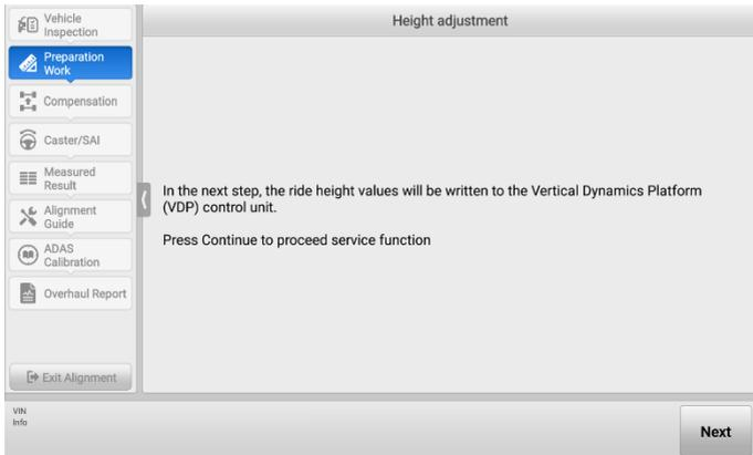
**Figure 4-28 Height Adjustment Screen 4**
