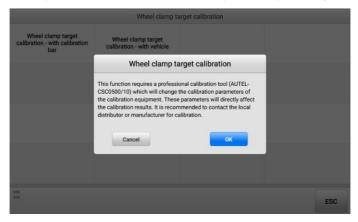
Figure 5-19 Select Calibration Method
