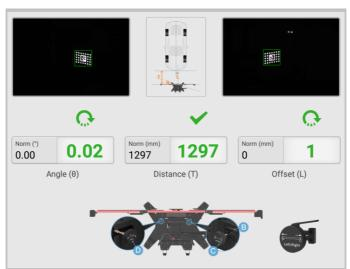
Figure 6-69 Adjust the Calibration Frame
