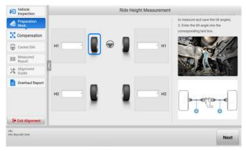
Figure 4-34 Measure and Input Tilt Angles
