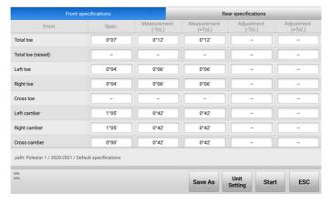
Figure 4-6 Edit Alignment Specifications Screen
