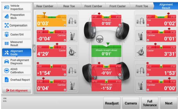
**Figure 4-57 Alignment Result Screen**
