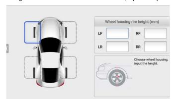
Figure 6-87 Input Wheel Housing Rim Height
