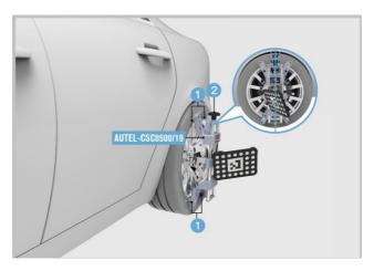
Figure 6-5 Install the Wheel Clamps (Rim Clamps)
