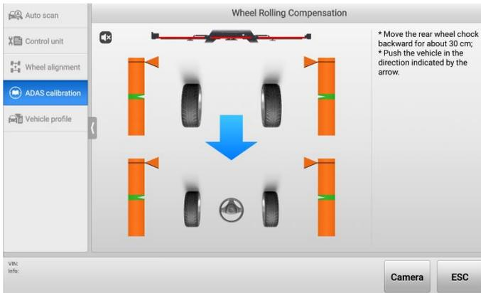
**Figure 6-40 Wheel Rolling Compensation 1**
