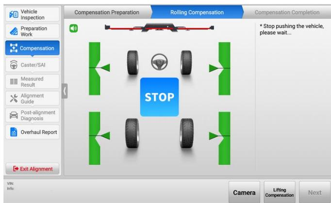
**Figure 4-37 Start Rolling Compensation 2 (Use Rim Clamp)**
