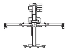
Figure 2-1 Calibration Frame AUTEL-CSC9000
