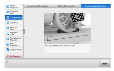
Figure 4-40 Complete Rolling Compensation (Use Rim Clamp)
