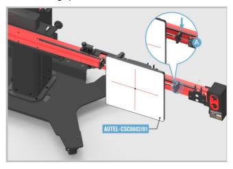
Figure 6-21 Adjust the Reflector 3
