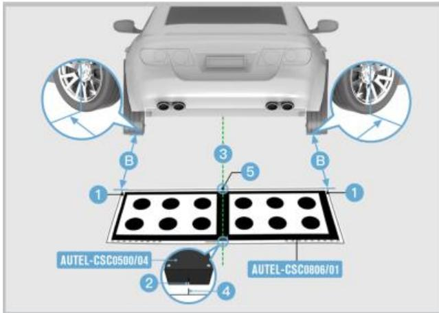
**Figure 6-53 Calibrate Camera Rear 1**
