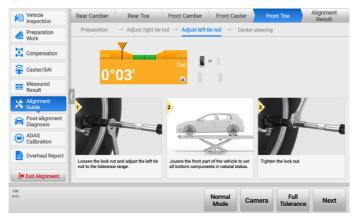
Figure 4-60 Adjust Left Tie Rod
