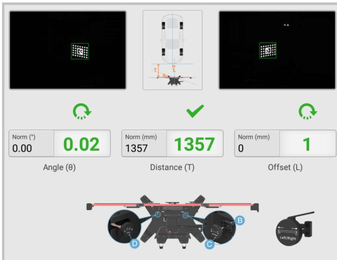
**Figure 6-7 Adjust the Calibration Frame**
