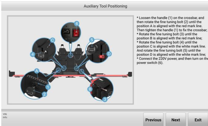
**Figure 5-52 Auxiliary Tool Positioning 2**
