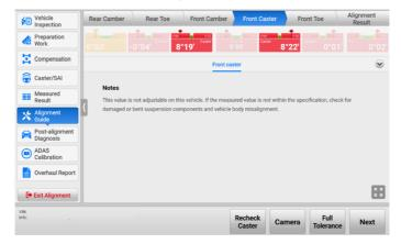
Figure 4-56 Parameters Adjustment Procedures Screen 2
