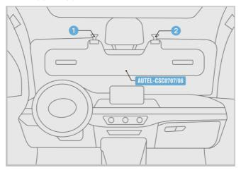
Figure 6-60 Place HUD Calibration Board
