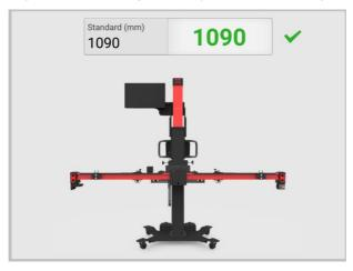
Figure 6-101 Adjust Standard Height
