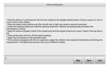
Figure 5-50 Vehicle Preparation Guide
