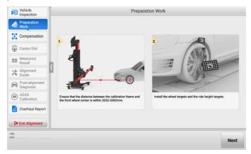
Figure 4-32 Install Ride Height Target
