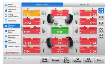
Figure 5-65 Measured Result (Half Tolerance) Screen
