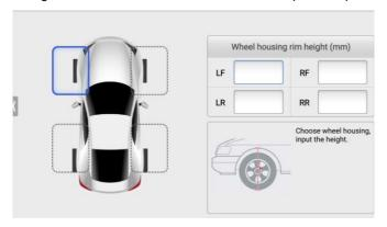
Figure 6-102 Input Wheel Housing Rim Height
