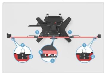
Figure 6-2 Position the Sliding Plate
