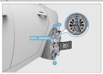
Figure 6-67 Install the Wheel Clamps (Rim Clamps)
