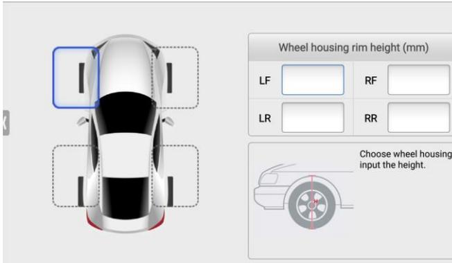
**Figure 6-102 Input Wheel Housing Rim Height**
