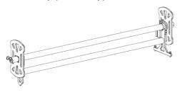
Figure 3-8 Calibration Bar — Suitable for Wheel Clamp (Rim Clamp)
