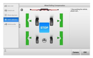
Figure 6-96 Wheel Rolling Compensation 4
