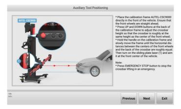
Figure 5-53 Auxiliary Tool Positioning 3
