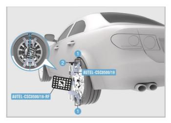
Figure 6-28 Install the Wheel Clamps (Rim Clamps)
