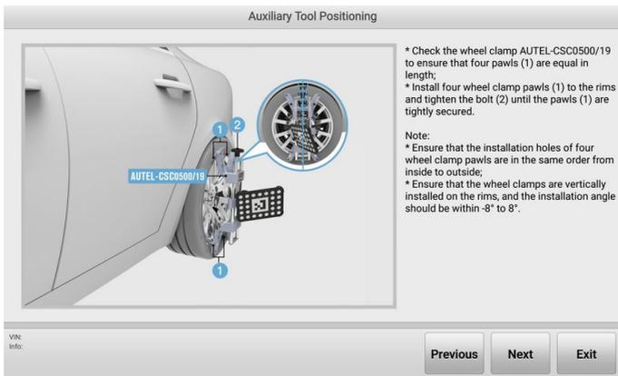
**Figure 5-45 Auxiliary Tool Positioning 4**
