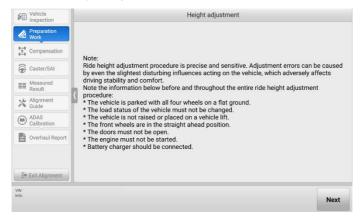
Figure 4-26 Height Adjustment Screen 2
