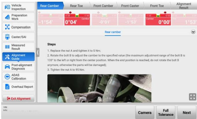
Figure 4-55 Parameters Adjustment Procedures Screen 1
