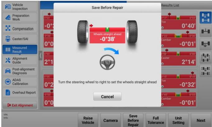
Figure 5-63 Save Before Repair Screen 1
