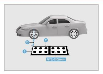
Figure 6-56 Calibrate Camera in Left Mirror 1
