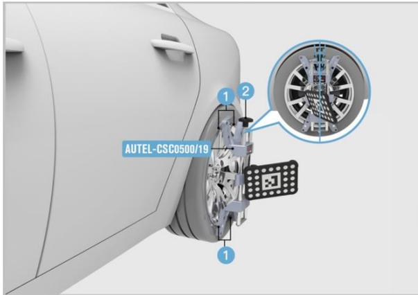
**Figure 6-92 Install the Wheel Clamps (Rim Clamps)**
