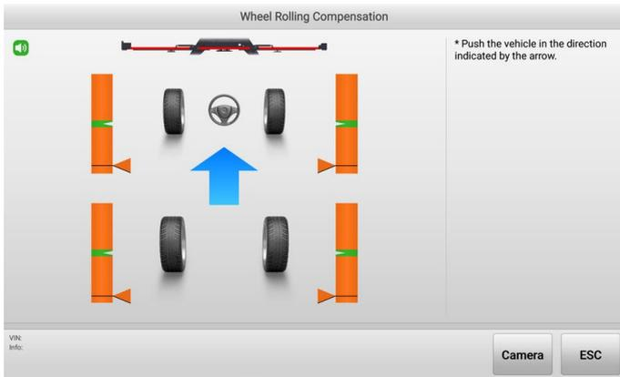
**Figure 5-48 Wheel Rolling Compensation 3**
