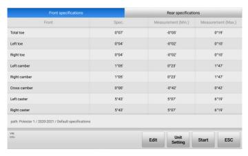
Figure 4-5 Alignment Specifications Screen
