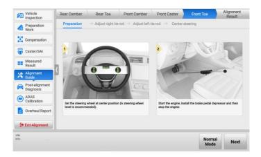
Figure 4-58 Front Toe Adjustment Preparation
