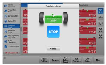
Figure 5-64 Save Before Repair Screen 2
