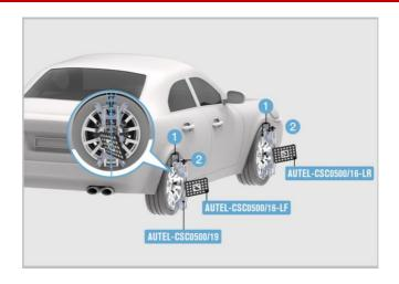
Figure 6-39 Install Wheel Clamps (Rim Clamps)
