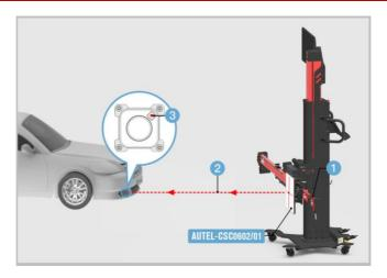
Figure 6-16 Align Laser with Mini Reflector
