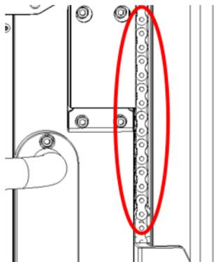
Maintenance method: locate the chain through the gaps on both sides of the calibration frame, and apply anti-rust oil along the surface of the chain.
