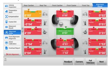
Figure 4-57 Alignment Result Screen
