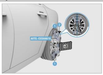
Figure 6-80 Install the Wheel Clamps (Rim Clamps)
