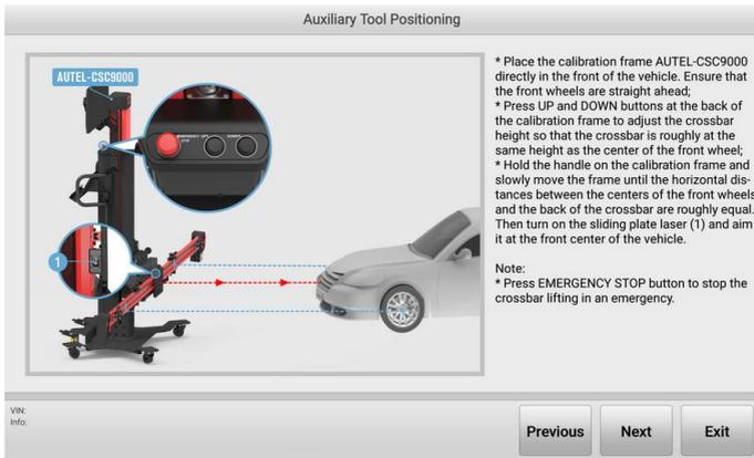
**Figure 5-53 Auxiliary Tool Positioning 3**
