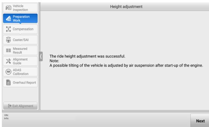
**Figure 4-29 Height Adjustment Screen 5**
