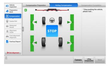
Figure 4-39 Start Rolling Compensation 4 (Use Rim Clamp)
