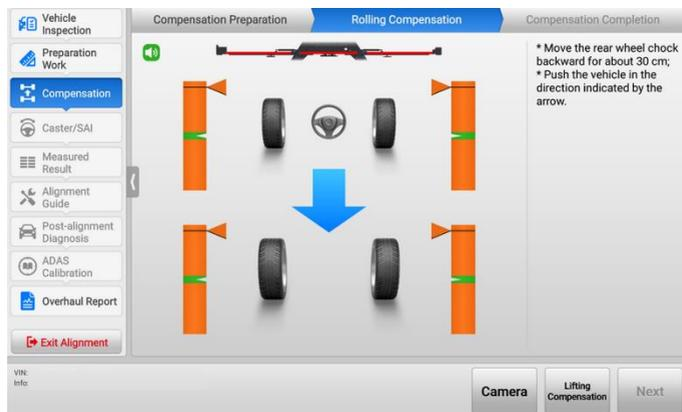
**Figure 4-36 Start Rolling Compensation 1 (Use Rim Clamp)**
