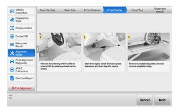
Figure 4-62 Recheck Caster Preparations
