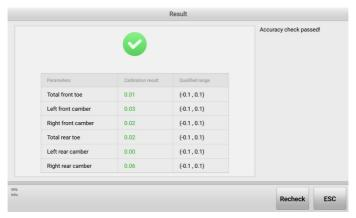
Figure 5-40 Accuracy Check Result Screen
