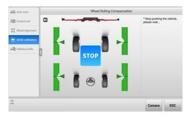
Figure 6-94 Wheel Rolling Compensation 2
