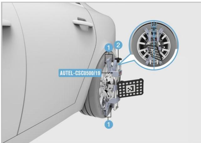
**Figure 6-80 Install the Wheel Clamps (Rim Clamps)**
