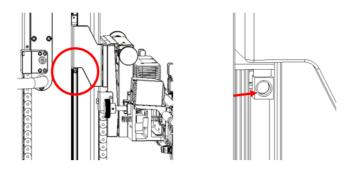
Maintenance method: locate the 2 oil filling ports (as the picture shows) from the gaps on both sides of the calibration frame and use a grease gun to fill them.
