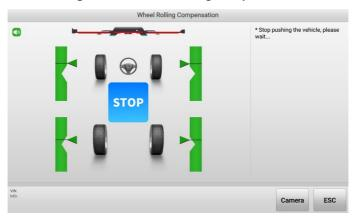
Figure 5-47 Wheel Rolling Compensation 2
