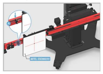
Figure 6-13 Adjust the Reflector 1
