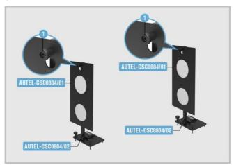
Figure 6-50 Mount the Target Board
