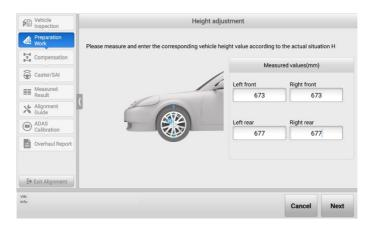
Figure 4-27 Height Adjustment Screen 3
