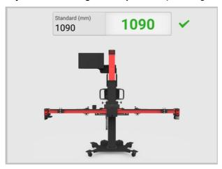
Figure 6-86 Adjust Standard Height
