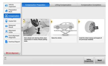
Figure 4-41 Lifting Compensation Preparation (Use Rim Clamp)
