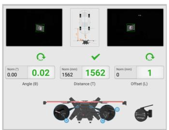
Figure 6-82 Adjust the Calibration Frame
