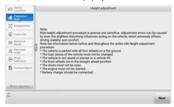
Figure 4-25 Height Adjustment Screen 1
