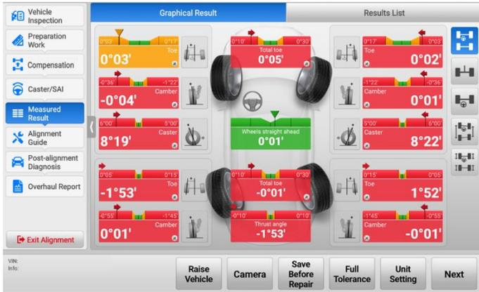
Figure 4-48 Measured Result Screen (Graphical Result)
