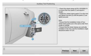
Figure 5-45 Auxiliary Tool Positioning 4
