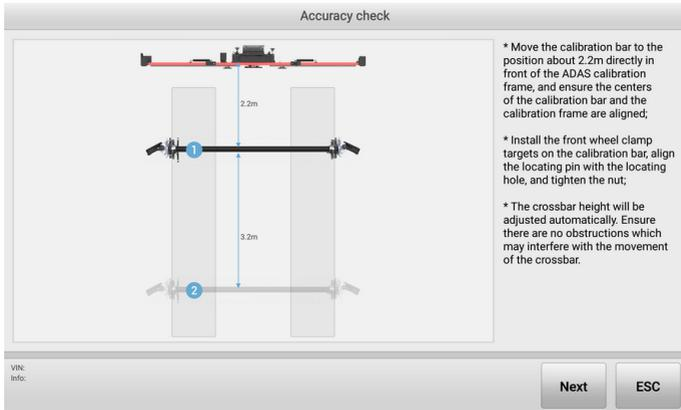
**Figure 5-35 Accuracy Check Screen (Use Calibration Bar) 1**
