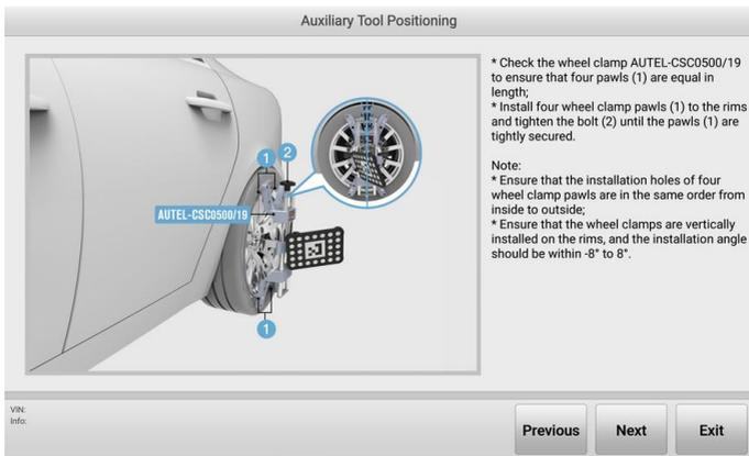
**Figure 5-54 Auxiliary Tool Positioning 4**
