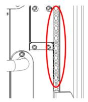
Maintenance method: locate the chain through the gaps on both sides of the calibration frame, and apply anti-rust oil along the surface of the chain.
