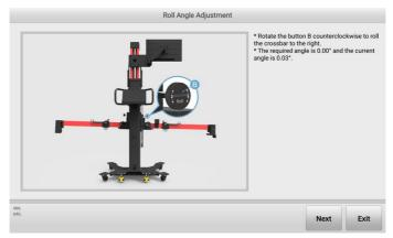
Figure 5-10 Roll Angle Adjustment 2
