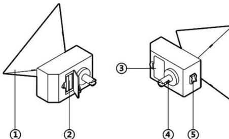
**Figure 3-18 Corner Reflector AUTEL-CSC0802/01**
