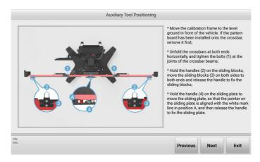
Figure 5-51 Auxiliary Tool Positioning 1
