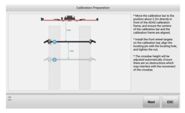
Figure 5-13 Aligner Calibration Preparation
