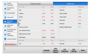
Figure 4-54 Measured Result Screen (Results List)
