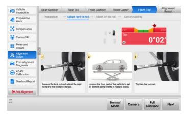
Figure 4-59 Adjust Right Tie Rod
