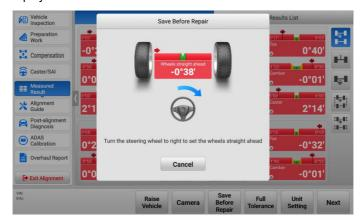
Figure 5-63 Save Before Repair Screen 1
