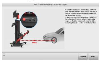
Figure 5-29 Calibration Preparation (Use Vehicle) 2
