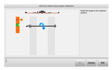
Figure 5-25 Start Calibration (Use Calibration Bar) 4
