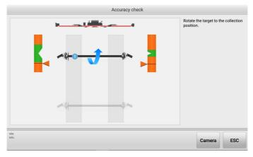
Figure 5-38 Accuracy Check Screen (Use Calibration Bar) 4
