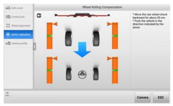
Figure 6-93 Wheel Rolling Compensation 1
