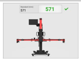
Figure 6-47 Adjust Standard Height
