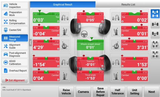
**Figure 5-66 Measured Result (Full Tolerance) Screen**
