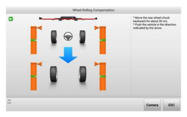
Figure 5-46 Wheel Rolling Compensation 1
