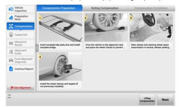
Figure 4-35 Rolling Compensation Preparations (Use Rim Clamp)
