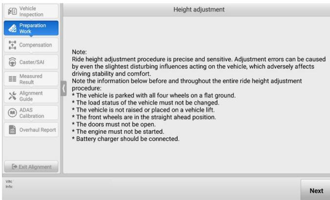
Figure 4-25 Height Adjustment Screen 1
