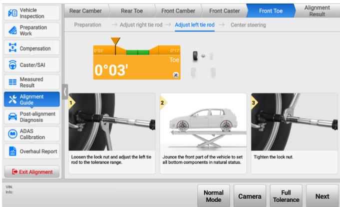
**Figure 4-60 Adjust Left Tie Rod**
