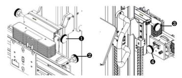
Figure 2-2 Fine-Tuning Mechanism
