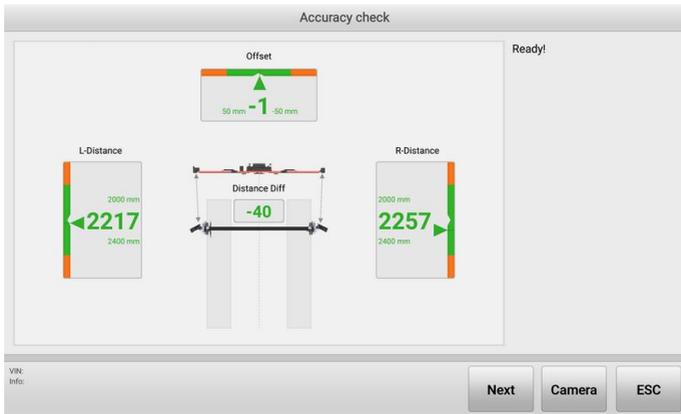
**Figure 5-37 Accuracy Check Screen (Use Calibration Bar) 3**
