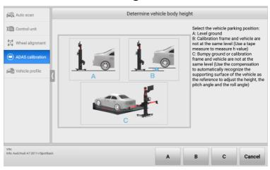
Figure 6-22 Select Vehicle Parking Position
