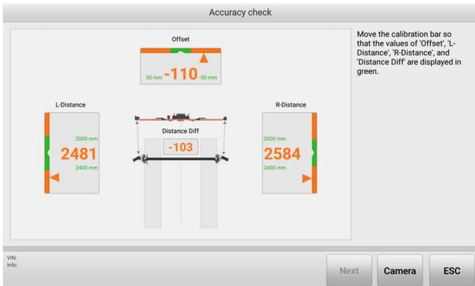
**Figure 5-36 Accuracy Check Screen (Use Calibration Bar) 2**
