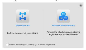
Figure 4-2 Wheel Alignment Function Entrance Screen
