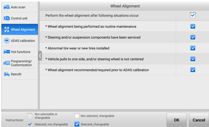
**Figure 4-12 Wheel Alignment Screen (Advanced Wheel Alignment)**
