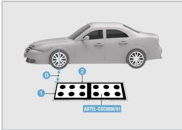
**Figure 6-56 Calibrate Camera in Left Mirror 1**
