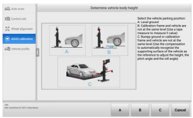
Figure 6-74 Select Vehicle Parking Position
