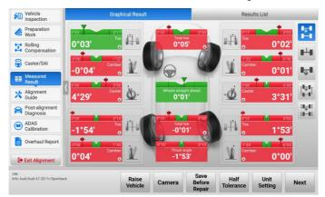
Figure 5-66 Measured Result (Full Tolerance) Screen
