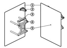
Figure 3-17 Radar Calibration Plate AUTEL-CSC0602/02
