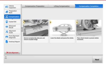
Figure 4-46 Complete Lifting Compensation (Use Rim Clamp)
