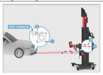
Figure 6-17 Align Reflected Laser with Origin Laser
