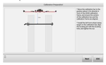
Figure 5-21 Calibration Preparation (Use Calibration Bar)
