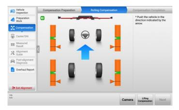
Figure 4-38 Start Rolling Compensation 3 (Use Rim Clamp)
