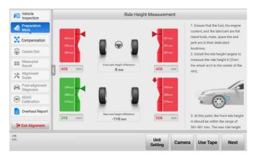
Figure 4-33 Measure Ride Height with Ride Height Target
