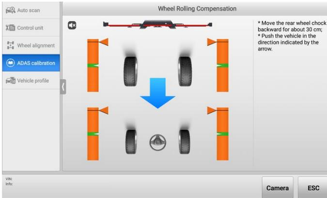
**Figure 6-93 Wheel Rolling Compensation 1**
