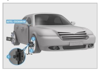
Figure 6-81 Adjust the Distance Measuring Target
