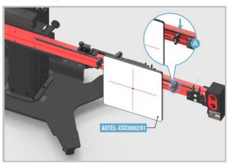
Figure 6-20 Adjust the Reflector 2
