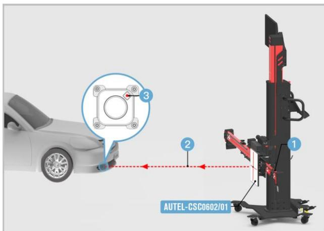
**Figure 6-16 Align Laser with Mini Reflector**
