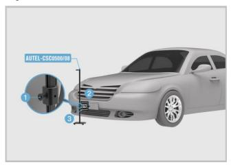
Figure 6-6 Adjust the Distance Measuring Target
