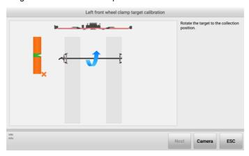
Figure 5-24 Start Calibration (Use Calibration Bar) 3
