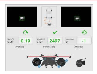
Figure 6-44 Position the Calibration Frame
