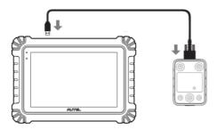
Figure 13-1 Connecting MaxiSys Tablet and Hand-held Inclinometer
