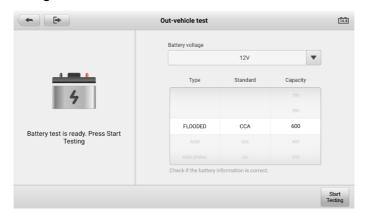
Figure 12-10 Out-vehicle Test Screen
