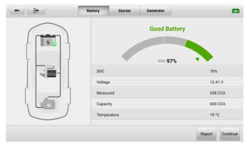
Figure 12-7 Battery Test Results Screen
