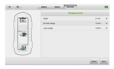
Figure 12-9 Generator Test Results Screen
