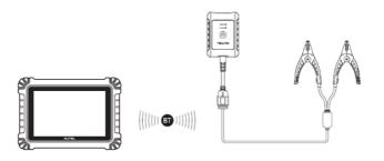
Figure 12-3 Battery Tester Connection Example 1
