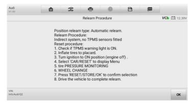
Figure 5-13 Relearn Procedure for Indirect TPMS
