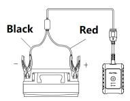
Figure 8-2 Connecting to a Battery
