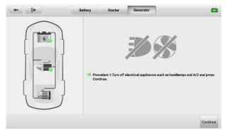
Figure 8-9 Generator Test Screen
