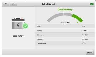
Figure 8-12 Out-vehicle Test Result Screen
