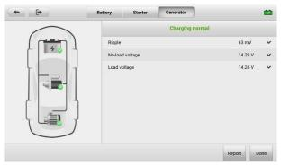
Figure 8-10 Generator Test Result Screen
