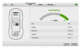
Figure 8-6 Battery Test Results Screen
