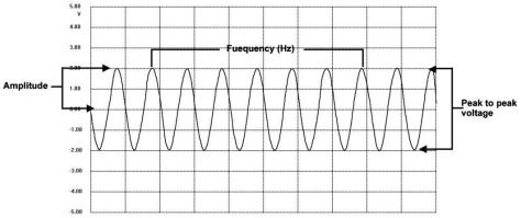
Figure 18-1 Sinusoidal Waveform
