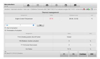
Figure 4-14 Active Test Screen
