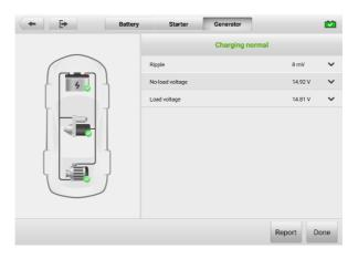
Figure 8-8 Generator Test Results Screen
