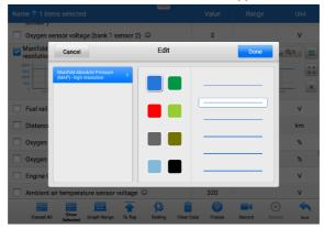
Figure 4-15 Waveform Edit Screen
