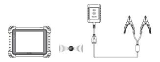
Figure 8-2 Connecting with the Tablet
