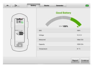
Figure 8-6 Battery Test Results Screen
