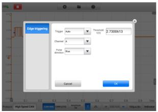
Figure 7-126 Trigger Settings Screen
