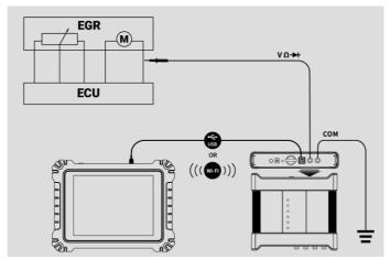
Figure 7-93 Actuator Drive Connection Diagram
