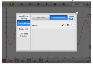
Figure 7-46 Probe Setting Screen (User-defined Probe)
