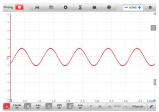
Figure 7-48 After Setting Low-pass Filtering Screen
