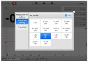
Figure 7-77 Amplitude Setting Screen (DC 2.0 V/div)
