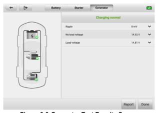
Figure 9-9 Generator Test Results Screen
