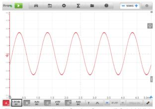
Figure 7-43 Amplitude Setting Screen (DC 1.0 V/div)
