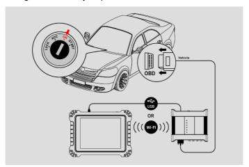
Figure 7-107 Connection Diagram
