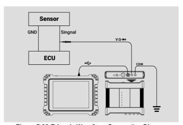
Figure 7-96 Triangle Waveform Connection Diagram
