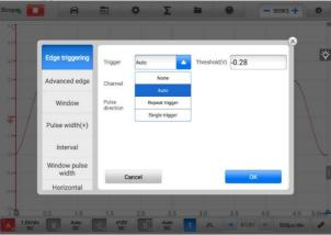
Figure 7-51 Trigger Mode Screen
