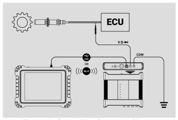
Figure 7-94 Square Wave Connection Diagram
