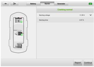
Figure 9-8 Starter Test Result Screen
