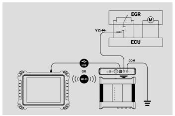
Figure 7-82 Connection Diagram
