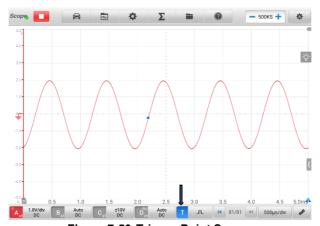
Figure 7-50 Trigger Point Screen
