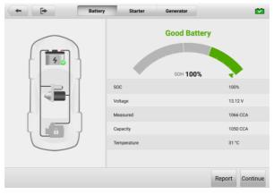
Figure 9-7 Battery Test Results Screen
