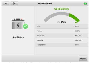
Figure 9-11 Out-vehicle Test Results Screen
