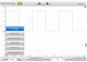
Figure 7-91 Signal Mode Setting Screen
