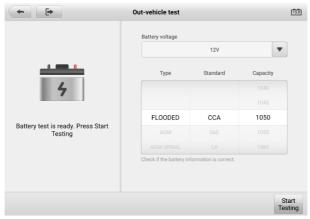
Figure 9-10 Out-vehicle Test Screen
