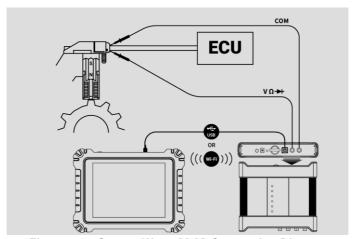
Figure 7-95 Square Wave (X+Y) Connection Diagram
