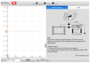
Figure 7-71 Wiring Diagram and Help Screen
