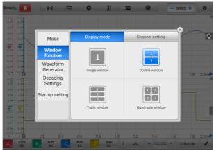
Figure 7-20 Display Mode Selection Screen
