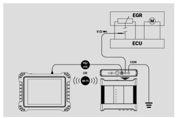
Figure 7-92 DC Voltage Connection Diagram
