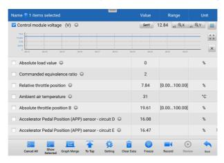
Figure 4-14 Waveform Graph Mode Screen
