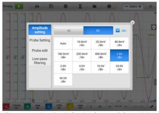
Figure 7-42 Amplitude Setting Screen (DC 1.0 V/div)
