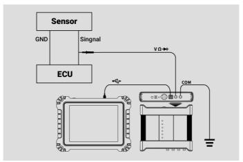
Figure 7-97 Arbitrary Waveform Connection Diagram
