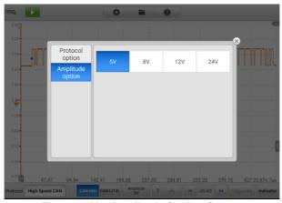
Figure 7-124 Amplitude Setting Screen
