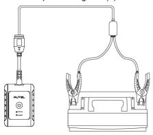
Figure 9-4 Battery Tester Connection Example 2
