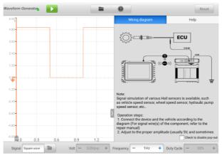
Figure 7-89 Wiring Diagram and Help Screen
