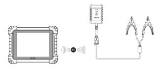
Figure 9-3 Battery Tester Connection Example 1
