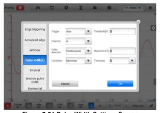
Figure 7-54 Pulse Width Settings Screen
