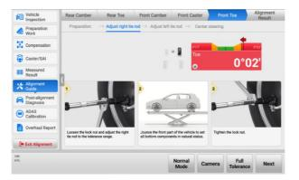
Figure 5-60 Adjust Right Tie Rod
