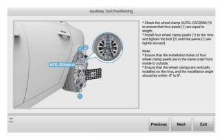
Figure 10-58 Auxiliary Tool Positioning 4
