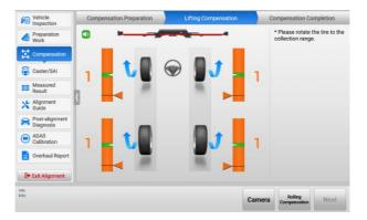
Figure 5-46 Start Lifting Compensation 4 (Using Rim Clamp)
