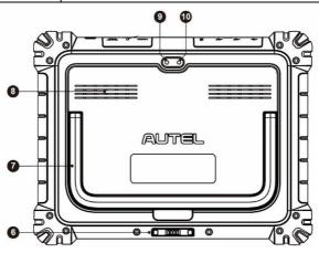
Figure 2-2 MaxiSys Tablet Back View
