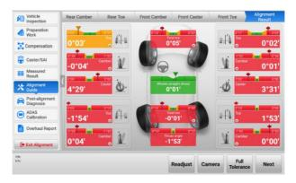
Figure 5-58 Alignment Result Screen
