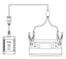
Figure 9-4 Battery Tester Connection Example 2
