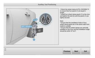
Figure 10-49 Auxiliary Tool Positioning 4
