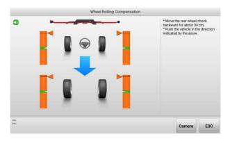
Figure 10-50 Wheel Rolling Compensation 1
