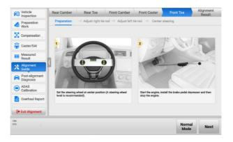
Figure 5-59 Front Toe Adjustment Preparation
