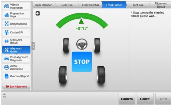
**Figure 5-64 Steering Wheel Adjustment**
