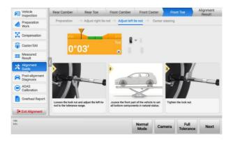
Figure 5-61 Adjust Left Tie Rod
