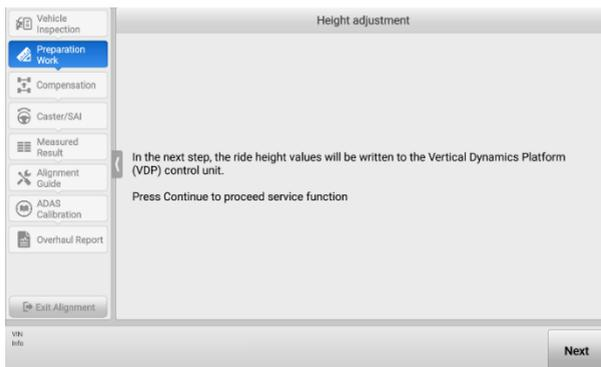
**Figure 5-29 Height Adjustment Screen 4**
