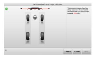
Figure 10-34 Start Calibration (Using a Vehicle) 1
