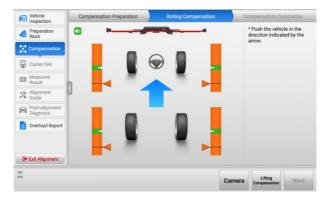
Figure 5-39 Start Rolling Compensation 3 (Using Rim Clamp)
