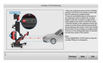
Figure 10-57 Auxiliary Tool Positioning 3
