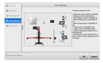
Figure 6-3 Prepare ACC Calibration Tools
