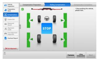
Figure 5-38 Start Rolling Compensation 2 (Using Rim Clamp)
