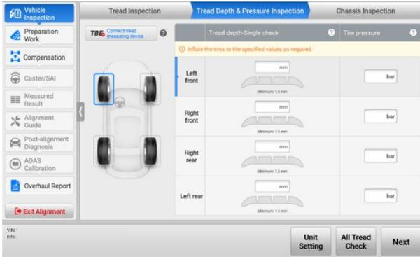
**Figure 5-16 Tread Depth & Pressure Inspection Screen 1**
