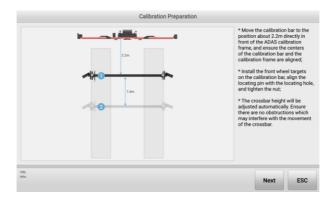
Figure 10-17 Aligner Calibration Preparation
