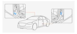
Figure 5-17 Standard Tire Pressure Value Location
