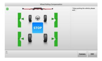
Figure 10-53 Wheel Rolling Compensation 4
