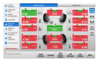
Figure 10-70 Measured Result (Full Tolerance) Screen
