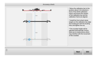
Figure 10-39 Accuracy Check Screen (Using a Calibration Bar) 1
