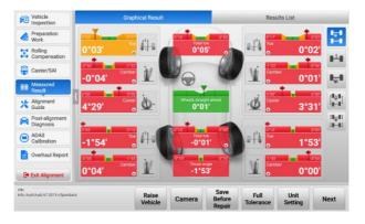
Figure 10-69 Measured Result (Half Tolerance) Screen
