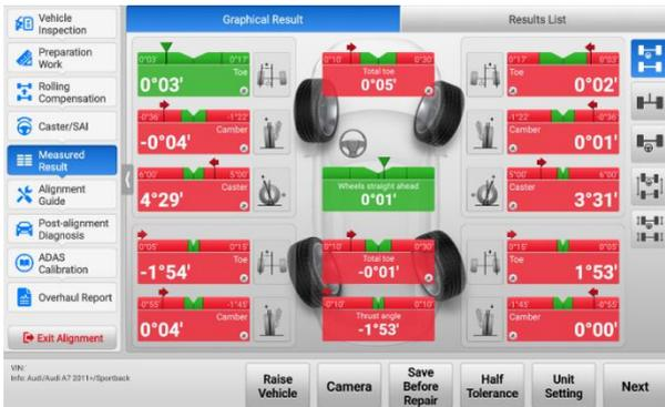
Figure 10-70 Measured Result (Full Tolerance) Screen
