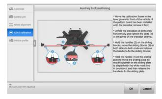
Figure 6-5 Position Auxiliary Tools for Calibration
