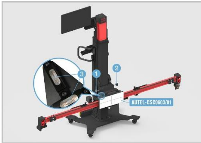
Figure 6-70 Center the Bubble Level of NV Calibrator
