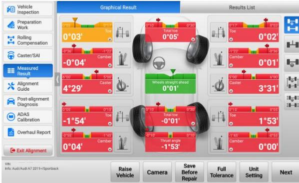
Figure 10-69 Measured Result (Half Tolerance) Screen
