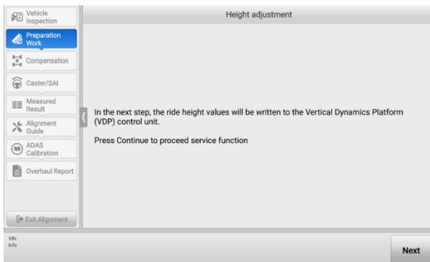
**Figure 5-29 Height Adjustment Screen 4**
