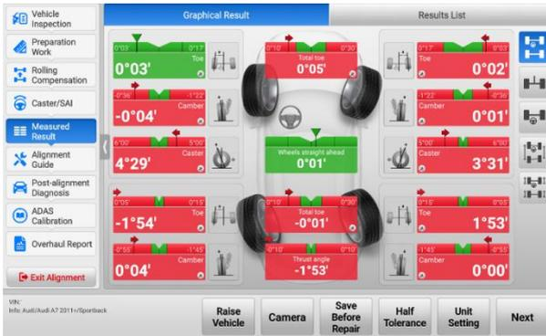
Figure 10-70 Measured Result (Full Tolerance) Screen
