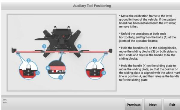
**Figure 10-46 Auxiliary Tool Positioning 1**
