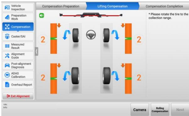
**Figure 5-45 Start Lifting Compensation 3 (Using Rim Clamp)**
