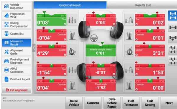
Figure 10-70 Measured Result (Full Tolerance) Screen
