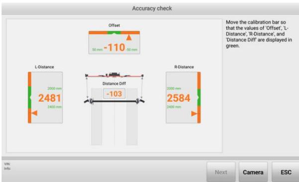
**Figure 10-40 Accuracy Check Screen (Using a Calibration Bar) 2**
