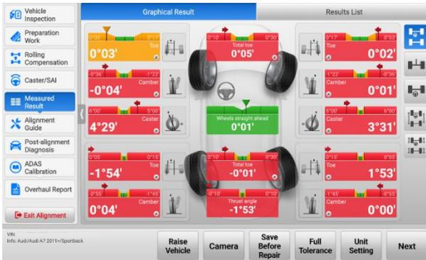
Figure 10-69 Measured Result (Half Tolerance) Screen
