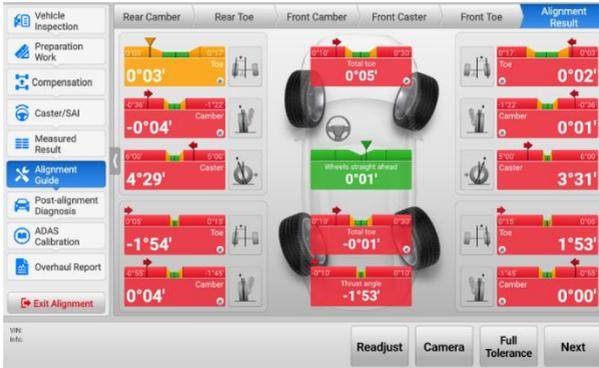
**Figure 5-58 Alignment Result Screen**
