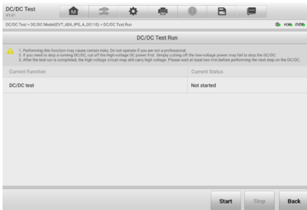
Figure 6-23 DC/DC Test Run Screen 1
