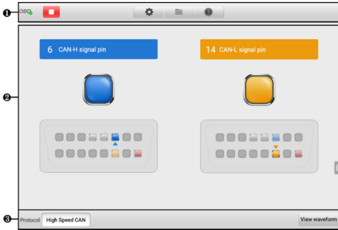
Figure 11-110 Bus Inspection Screen
