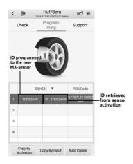
Figure 6-5 Programming Screen via OEM Part No.
