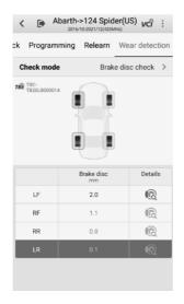
Figure 5-38 Brake Disc Check Screen
