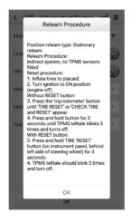
Figure 5-8 Relearn Procedure for Indirect TPMS
