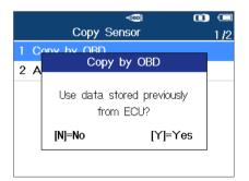
Press Y to use the previously stored data, and then the sensor IDs saved in the ECU displays; or press N to use new data, and then the following screens display.
