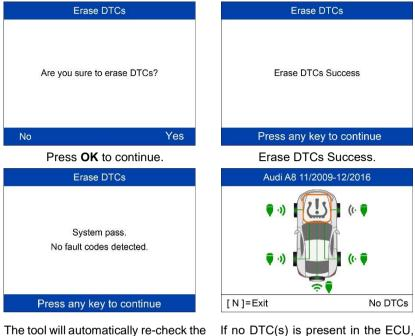
The tool will automatically re-check the ECU to ensure all DTCs have been deleted.
