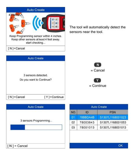
Once the sensors are successfully programmed, the sensor IDs and the PSNs (Product Serial Number) will display on the tool.
