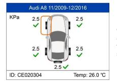
Once all sensors are successfully activated, the tool will prompt users to perform OBD Relearn, if supported by the vehicle.
