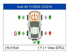
Use Up and Down Arrow button to select the TPMS icon in the center of the graphed vehicle and press **Y** to view the DTCs.
