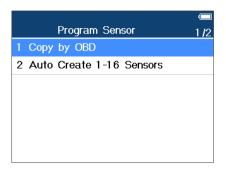
There are two ways to program MX-Sensors: Copy by OBD and Auto Create 1-16 Sensors.
