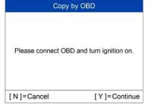
Follow the onscreen instructions to connect the tool with the test vehicle via the OBD II cable. Press **Y** to continue, or press **N** to exit.
