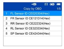
The sensor IDs saved in the ECU display on the screen.
