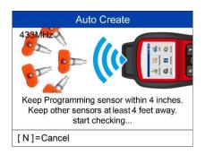
The tool will automatically detect the sensors near the tool.
