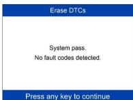
The tool will automatically re-check the ECU to ensure all DTCs have been deleted.
