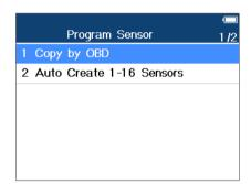
Press Y to confirm selection. If no TPMS diagnosis is performed before, the tool will prompt the user to connect OBD cable and then read information from the ECU. If TPMS diagnosis is performed, then the next screen displays.
