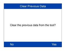
If sensor activation is performed and there is data saved in the tool, a Clear Previous Data message displays. Press **No** to turn to the existing sensor activation menu and reactivate one sensor, then the tool will prompt you to connect OBD cable for ECU diagnosis, or press **Yes** to clear the previous data and reactivate the sensors.
