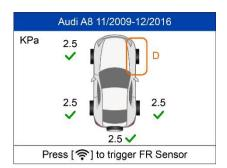
All sensors have been triggered. Display advances to connect OBD cable for diagnosis even if not all sensors have been successful activated.
