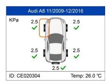
Once all sensors are successfully activated, the tool will prompt users to perform OBD Relearn, if supported by the vehicle.
