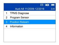
If there is sensor triggered, the tool will ask whether to clear the saved data, press **N** to use the saved data and reactivate one sensor, the tool will instruct you to connect OBD cable and then perform OBD Relearn; or press **Y** to clear the data and display the Relearn Procedure. The Relearn Procedure displays when no sensor is triggered.
