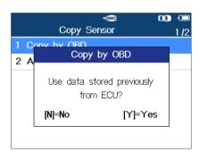
Press Y to use the previously stored data, and then the sensor IDs saved in the ECU displays; or press N to use new data, and then the following screens display.
