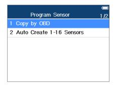
There are two ways to program MX-Sensors: Copy by OBD and Auto Create 1-16 Sensors.
