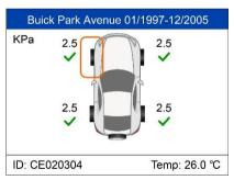
Once all sensors are successfully activated, then follow the Relearn Procedure to perform Stationary Relearn.
