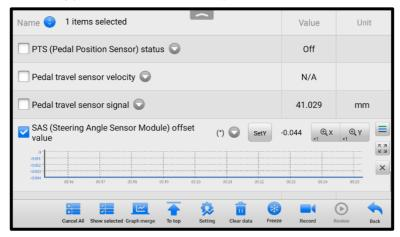
Figure 5-11 Waveform Graph Mode Screen
