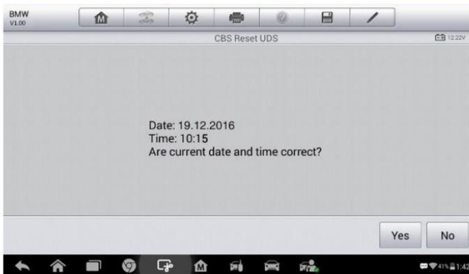
**Figure 7-2 Sample Oil Reset Service Screen 1**
