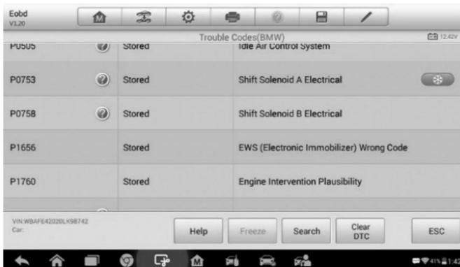
**Figure 6-7 Sample DTC & FFD Screen**
