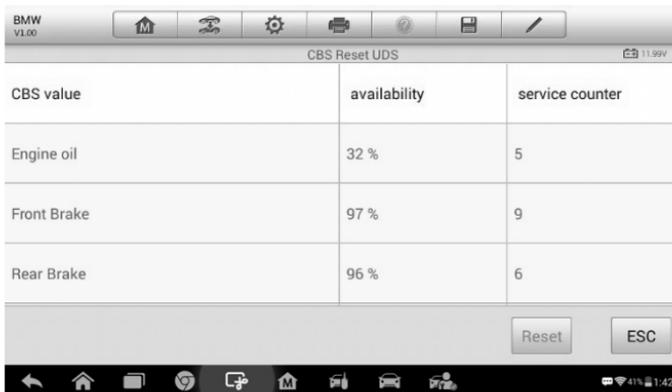
**Figure 7-3 Sample Oil Reset Service Screen 2**
