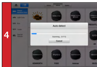
4 - Once the vehicle is successfully identified, the Diagnostics Menu will appear.
