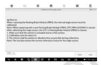
Figure 7-5 Sample Calibration of the Angle Sensor Screen 1
